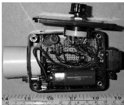
Bulb Firer with hotfoot connection, manual fire button, bulb isolation / on switch, power on LED and bulb correctly seated LED
