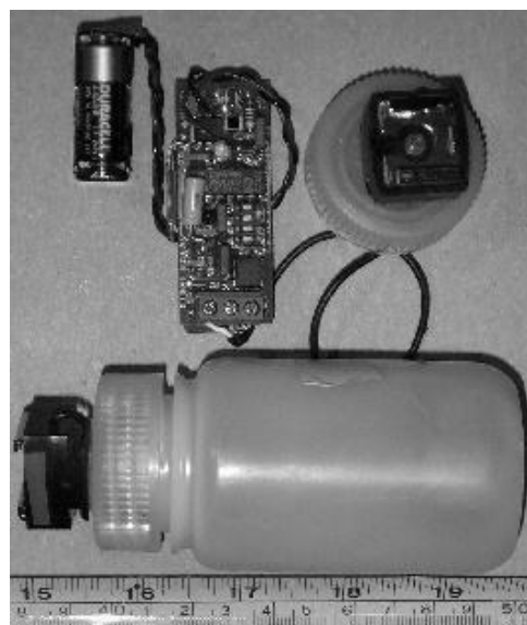
RALF Unit, housed in Nalgene bottle, complete with hotfoot connector
